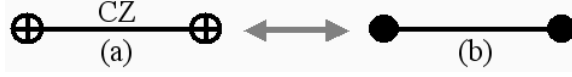
Figure 7: The two-vertex graph state is generated (a) by initializing each qubit in the |+\rangle state and then operating with a CZ gate, yielding (b).
